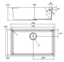
All dimensions are approximate only and are subject to change by the manufacturer. Bench cut-outs should not be undertaken based on these dimensions
