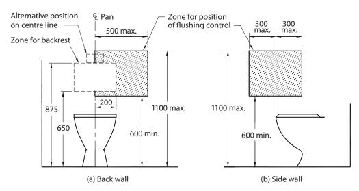
DIMENSIONS IN MILLIMETRES ZONE FOR POSITION OF FLUSHING CONTROL
