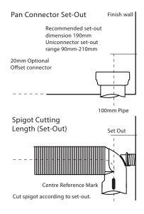
**3.** Cut height for 180mm and pan connection end 195mm from the wall.
