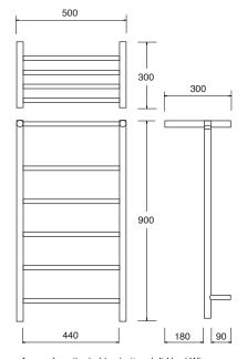
As you face the ladder, bottom left Hard Wire (50mm from the bottom of the rail).
