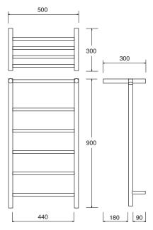
As you face the ladder, bottom left Hard Wire ( 50mm from the bottom of the rail ).
